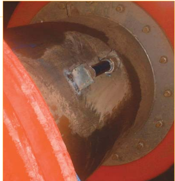
The Roxby transmitter was fitted inside 2 machined housings and these were welded to the side of the QServ Gauge PIG.
