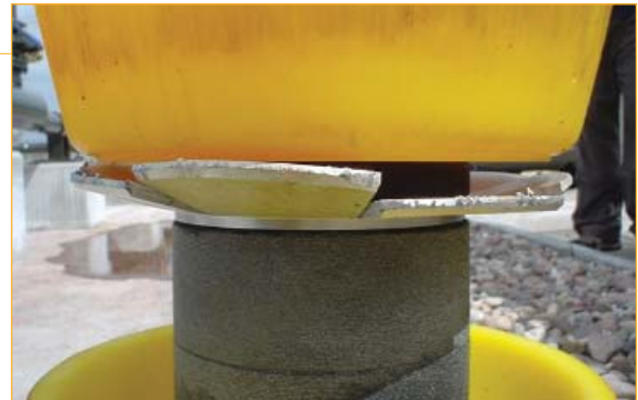
Gauge PIG with damaged gauge plate indicating that some blockages were apparent
